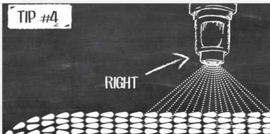
Take control with proper nozzle placement. Are you spraying just the grain, or are you spraying all over your equipment, too, due to haphazard nozzle placement? Test the direction and formation of your spray pattern as you begin, and make adjustments as necessary to avoid poor coverage or wasted product.
