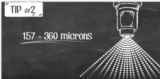
During product application, droplets should be at least 157-360 microns; coarse or very coarse droplets.
